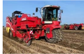
Two-row harvesters capable of harvesting two planted furrows simultaneously.
