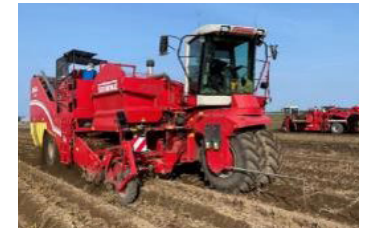
Two-row harvesters capable of harvesting two planted furrows simultaneously.
