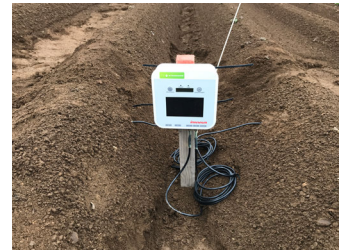
Soil moisture meter installed in a potato field
