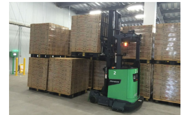
Unmanned forklift trucks (Kyoto Plant)
