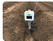
Soil moisture meter installed in a potato field
