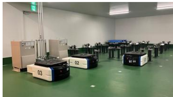
Raw materials and packaging materials transported by Automated Guided Vehicles (AGVs)
